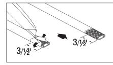
Place heat shrink tube over cable and leave %" of the tube hanging off the cable. Heat shrink the tube and while still hot, use pliers to pinch overhang together to seal end; hold for 15 seconds.
