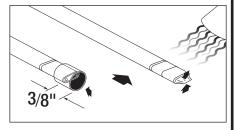
3. Place heat shrink cap over the sealed end and heat shrink until inner sealant starts to appear from the cap edge.
